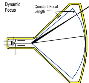
The optimum focal length for the beam varies as the beam scans from top to bottom and from side to side on the face of the CRT leading to a difference in focus between the centre and edges of the screen.
