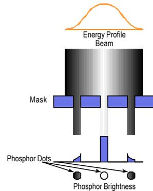
The subjective sharpness of a display is strongly affected by the focus of the monitor. This is an extremely difficult factor to measure and there is no industry-wide agreement on a simple number that can be used to summarise the performance of a display. (Note that the focus of a monitor should not be judged until it has warmed up for 20/30 minutes - see page 14).
