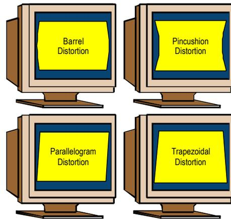
Because of their reliance on magnetism, screen images are affected by the direction that the monitor is facing (see page 13). As the monitor is rotated through the earth's magnetic field, changes in tilt can occur. Some monitors have user adjustments to compensate for this, while others have built in magnetometers and digital circuitry to eliminate the effect.
