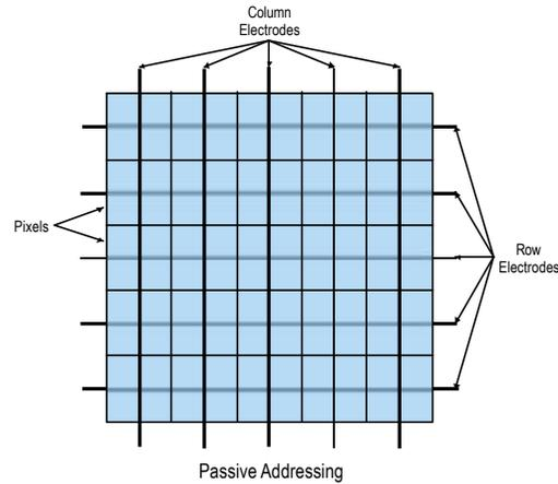
When a row is selected, the appropriate voltages are fed to individual column driver circuits. Current flows through the column lines to the selected row and the LC materials align accordingly. The drive circuits then move to the next row and repeat the operation. When the scanned row reaches the bottom of the display, it starts again at the top of the display.
