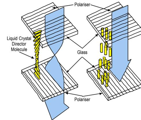
The screen is divided up into picture elements (pixels). The image is built up using these pixels. In a colour LCD, each pixel is fitted with either a Red, Green or Blue filter.
