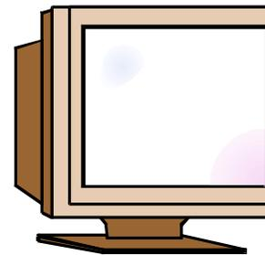
Because monitors are so sensitive to tiny fluctuations in magnetism, each time a monitor is switched on a 'degauss' operation is performed; that is to say, a coil fitted around the front of the CRT is used to 'extract' any residual magnetism from the shadow mask. If the monitor is subsequently moved or rotated, the influence of the earth's magnetic field will be different and this may result in colour patches.
