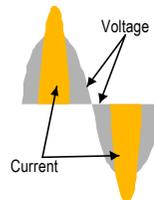
supplying devices such as heaters and lamps, do not absorb power evenly through the mains cycle. This can lead to power waste and problems in power generation, so legislation is likely to insist on power factor correction in the future.
