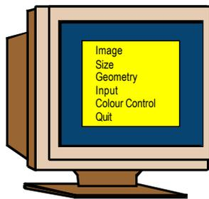
and because it is possible to make the screen display worse by bad setting, some manufacturers offer the facility to lock all but the most common brightness and contrast controls. A special sequence may be used to unlock the controls for service or support purposes.
