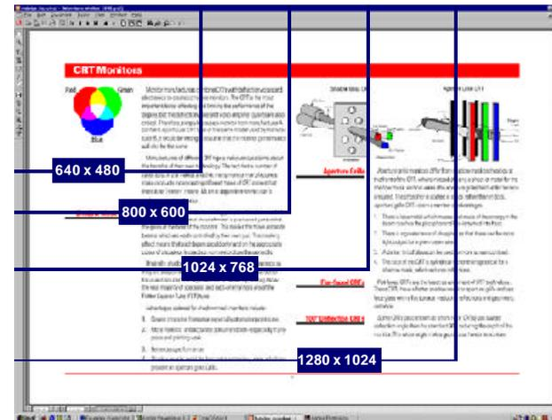
as many software packages use text that is limited to a fixed number of dots. If this software is used on a small screen with high resolution, the text may be too small for you to view comfortably. On the other hand, simply increasing the size of the monitor will not necessarily improve the image on the screen, unless the resolution is also increased. Sometimes a larger screen simply makes the characters and images more 'dotty'.
